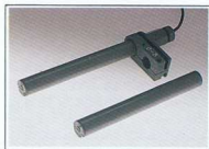
HH-3 Probe with C-3 Clamp and Replacement Probe Barrel MB-3.
